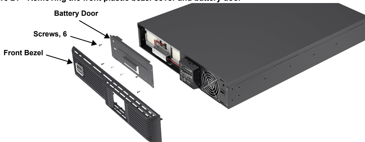
Figure 21 Removing the front plastic bezel cover and battery door
